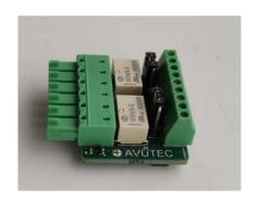
The IO extender is a level shifter and relay-board in one, that is used as an extender of the IO pins in the back of all Gatekeeper-X models. It is used to generate a Wiegand signal and communicate with electronic devices via relais.
